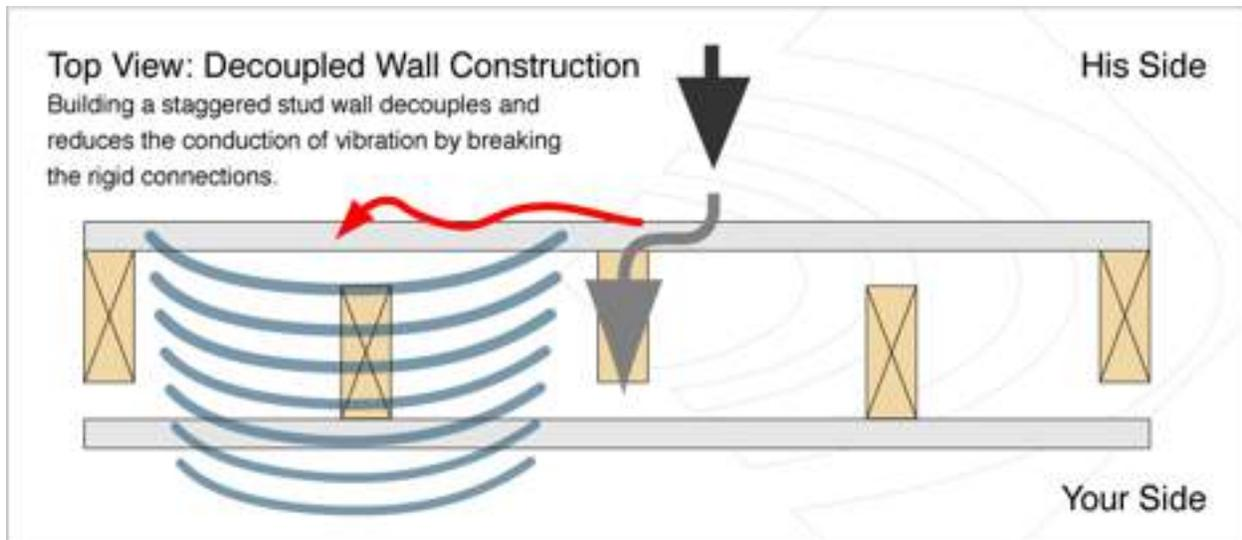
We can see how decoupling the wall studs limits the vibration trying to conduct through the wall. We are left with the airborne transmission represented by the blue waves. Note how decoupling does not affect airborne transmission.
